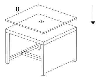
Do not fully tighten bolts until assembly is complete
